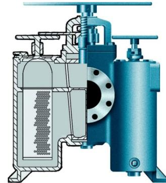
The plug diverting style also utilizes a casting consisting of two strainer basket chambers and between them, a diverting valve.
