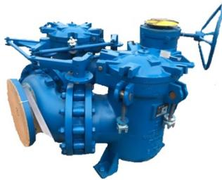
Although it is possible to use ball valves for flow diversion, resilient seated butterfly valves are compact and are less costly. This style of duplex strainer is only available with cast iron bodies and therefore most applications involve water, so complex ball valves or double/triple offset butterfly valves are not required.
