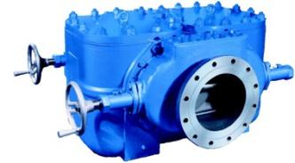
The isolation valves are mounted to screws and slide along rails cast into the strainer body when the handwheel is rotated. There are two valves and handwheels which are connected by a chain drive, so operating one handwheel moves both inlet and outlet valves simultaneously.
