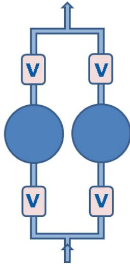
If you are using four valves (one for each strainers' inlet and outlet), the operator needs to operate each of the valves in a specific order to ensure uninterrupted flow.
